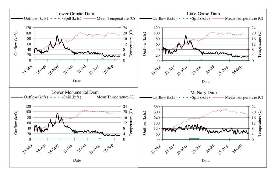
Figure 8. Measurements of outflow, spill, and mean temperature at Lower Granite Dam (top left), Little Goose Dam (top right), Lower Monumental Dam (lower left) and McNary Dam (lower right), from April 2 to September 2, 2001. Data was obtained on line at <a href="http://www.cqs.washington.edu/dart">http://www.cqs.washington.edu/dart</a>.
